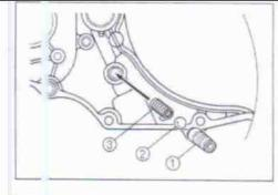
Install the spring ③, oil check valve ball ② and bushing ① to the right crankcase as shown.
